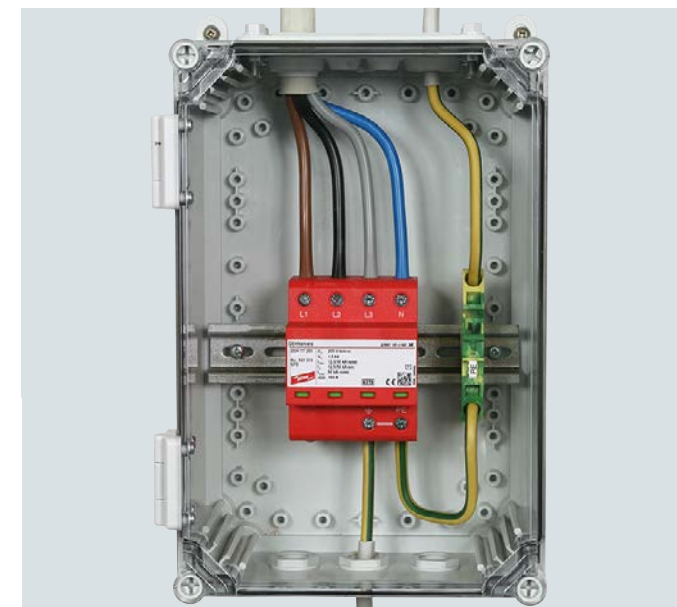
For protecting compact low-voltage consumer's installations against surges and even direct lightning strikes. For installation in conformity with the lightning protection zone concept at the boundaries from 0_A - 2 .
