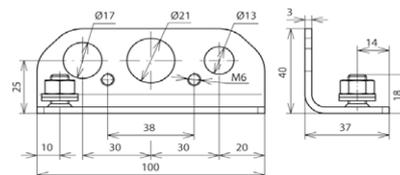
With three mounting boreholes for three different sizes of DEHNgate arresters, e.g. 1x 929 042 + 1x 929 057 + 1x (929 043, 929 044, 929 045 or 929 059).
