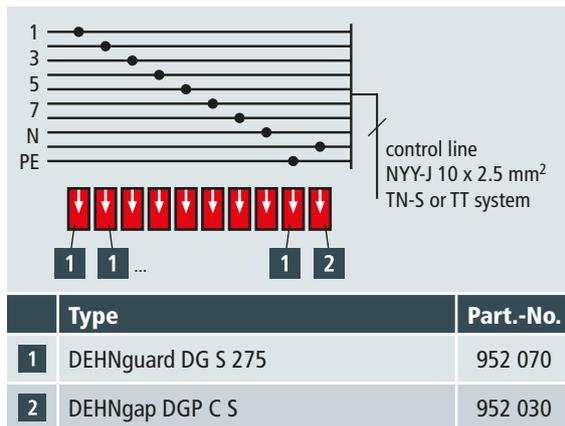
Figure 2 Example of surge protective devices for the bell controller
