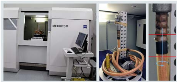
Figure 7 Test setup for the 3D computer tomography (red: measuring range, blue: axis of rotation)
