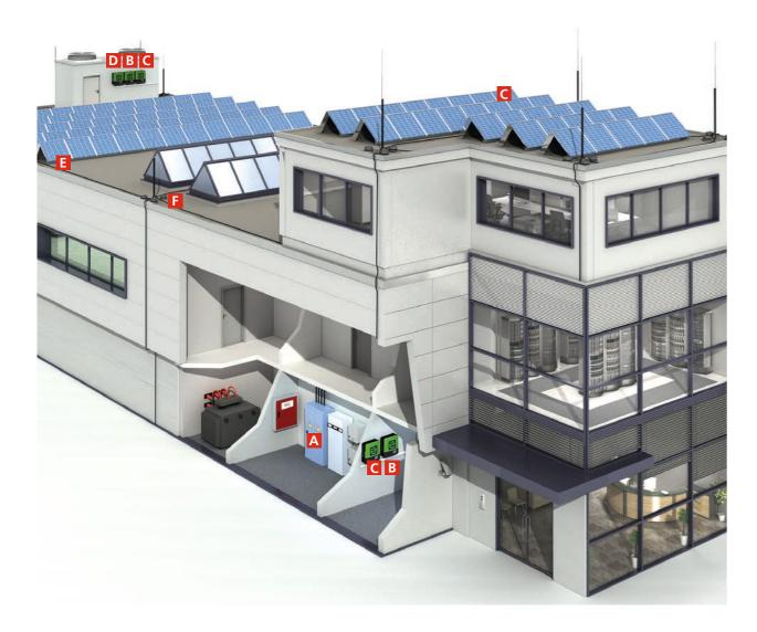
The PV modules must be located in the protected volume of the isolated air-termination system – whilst also maintaining the separation distance "s".
