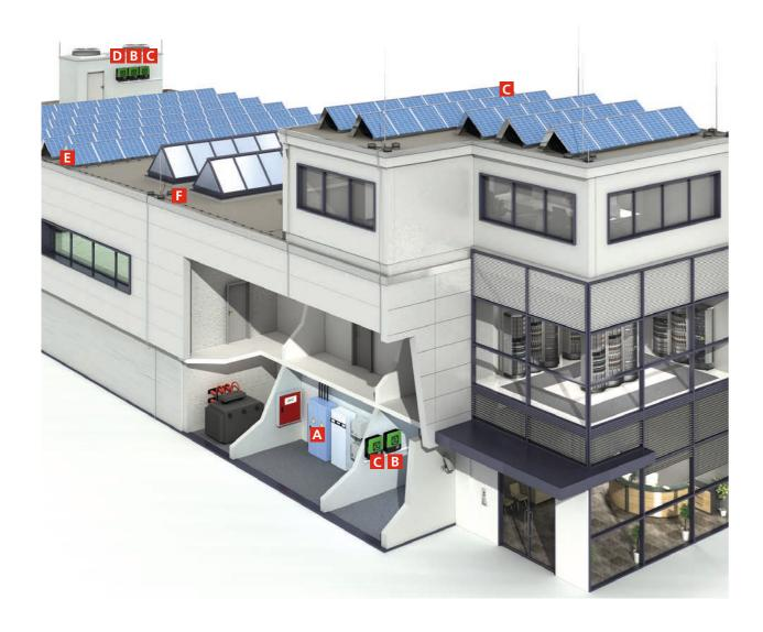
If the separation distance "s" cannot be maintained, lightning equipotential bonding is required.
