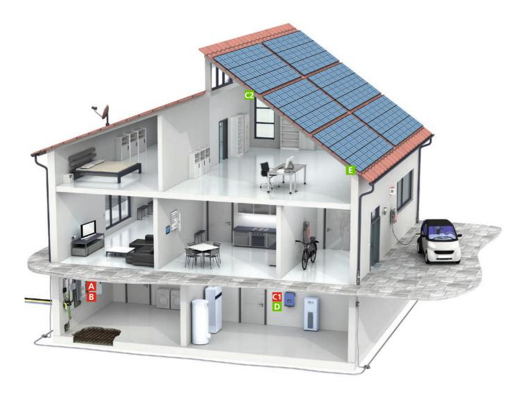
Surge protective devices should be installed even if there is no external lightning protection system.
