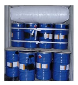
• In the final row it is essential that the last packing units loaded in the container are secured in such a way that they do not put pressure on the inside of the door of the container (danger when opening the door to unload) – see diagram
