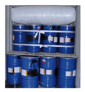
• In the final row it is essential that the last packing units loaded in the container are secured in such a way that they do not put pressure on the inside of the door of the container (danger when opening the door to unload) – see diagram
