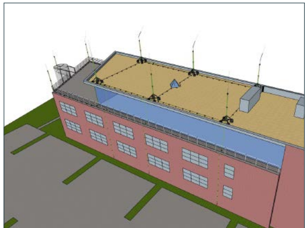
Positioning of the air-termination systems
