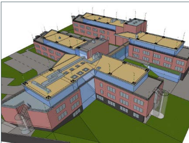
Positioning of the air-termination systems
