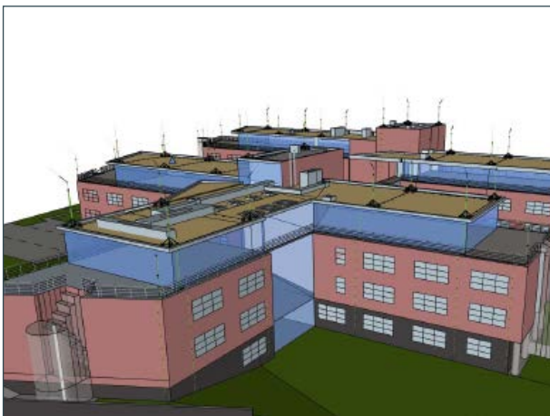
Positioning of the air-termination systems
