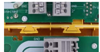
Side-by-side mounting of several devices thanks slide-in dovetail connections on the enclosures (DBX TC B 180).
