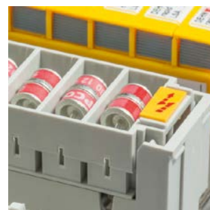
Pluggable surge arresters in the form of protection magazines can be plugged into terminal or disconnection blocks.
