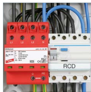
Series connection by means of a lightning-current-tested STAK 25 pin-shaped terminal
