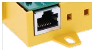
RJ45 socket at the output for direct connection to the router (DBX TC B 180).
