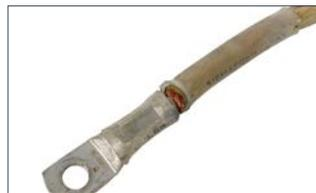
Bare strand protrudes from the broken cable entry.
