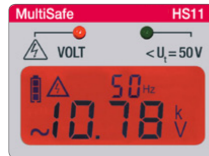
Colour change of the display at voltage
