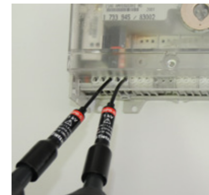
Flexible pin prods for tight contacts
