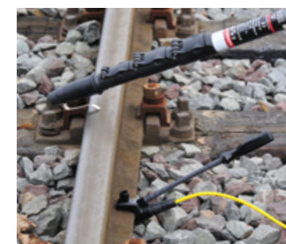
Fast self-test for device function and contact between terminal and rail MultiSafe TT 3K - with rail foot clamp
