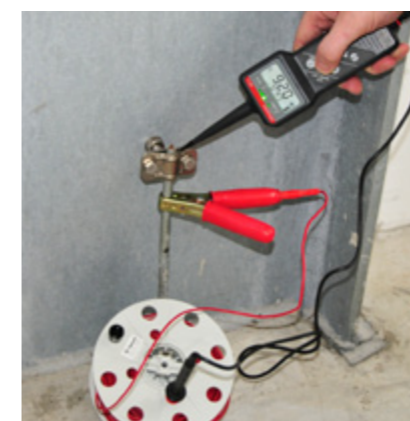
Quick compensation of the measuring line
