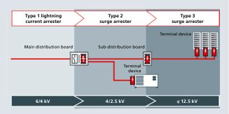
Interaction of the individual protection stages ensures the best possible protective effect. To this end, the relevant arresters must be energy coordinated according to IEC 60364-5-53 clause 534.
