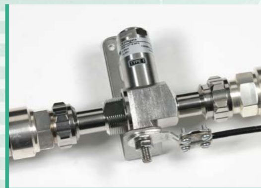
Befestigung des DEHNgate Art.-Nr. 929 146 mittels Erdungsschraube am Befestigungswinkel Art.-Nr. 106 310 und am Erdungskabel Art.-Nr. 416 411 Fixing of DEHNgate Part No. 929 146 with earthing screw at the angled fixing plate Part No. 106 310 and at the earthing conductor Part No. 416 411
