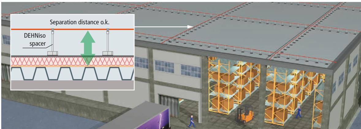
Figure 6 Elevated air-termination system to observe the separation distance
