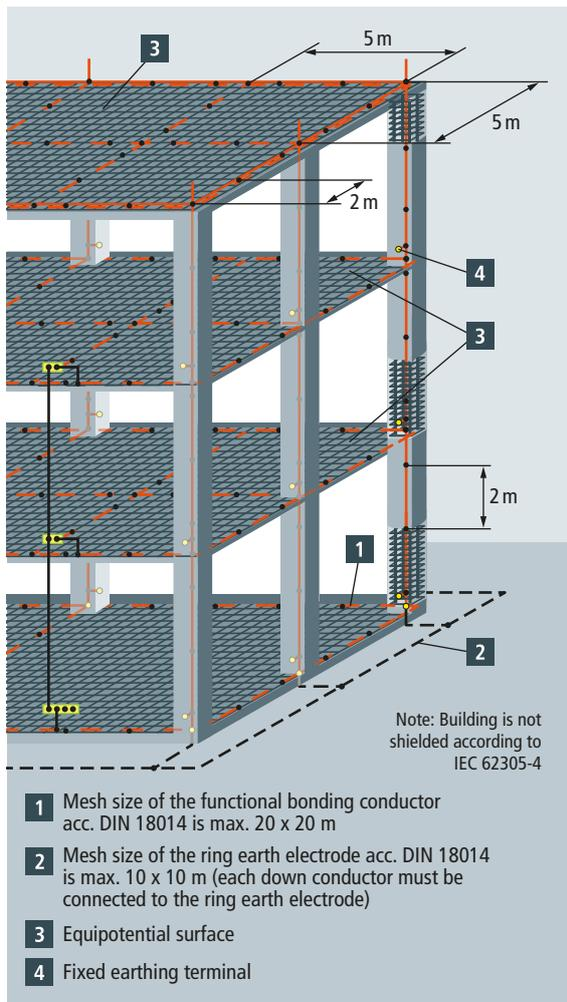
Figure 2 Building with equipotential surfaces and air-termination system (optional e.g. for curtain wall)
