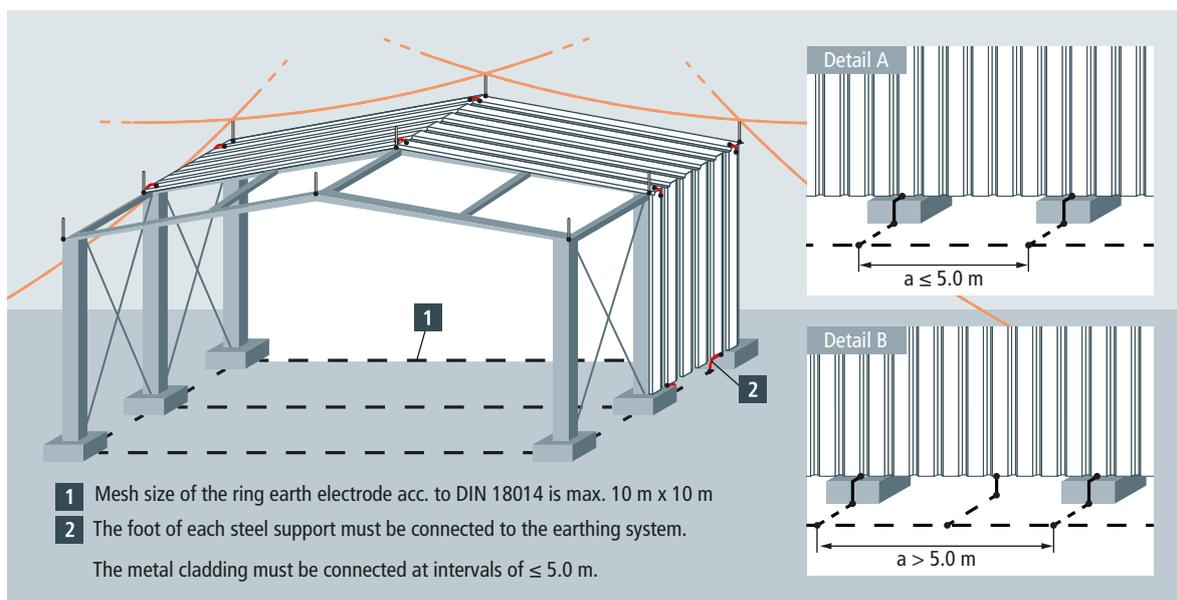
Figure 5 Steel hall with continuous metal cladding
