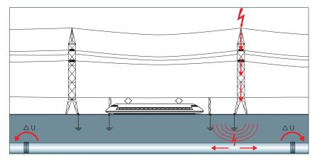
All these interference voltages may cause personal or material damage and a.c. corrosion.
