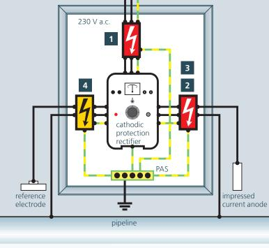
Protection solution for protective currents between 12 A and 60 A
